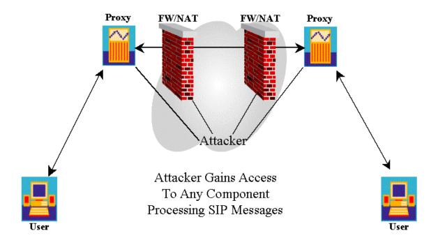
SIP messages have no built-in means to insure integrity. By manipulating SIP messages, an attacker can execute the same types of attacks described for registration hijacking and proxy impersonation.
