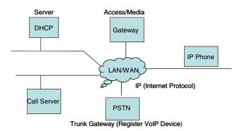
Figure 4: VoIP and IP-based LAN/WAN topology
