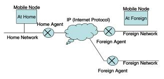
Figure 3: Typical Mobile IP topology
