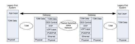
Figure 3 CES protocol encapsulation
