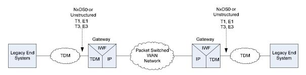
Figure 2 Reference model for CES over IP
