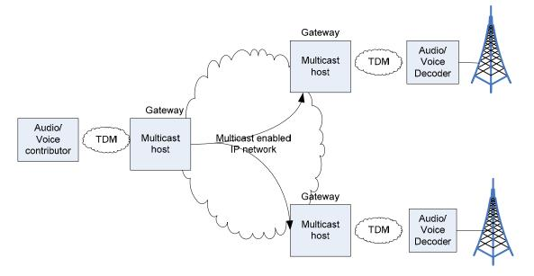
Figure 6 Integrated Multicast host
